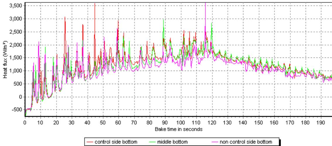
The bottom heat profile also exhibits some cross-band variation. This appears to affect the non-control side in particular after 60 seconds of the 190 second bake.
