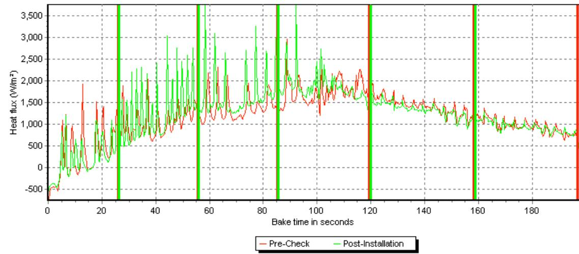
As one of the targets was to improve the base colour most of the extra heat was applied to the bottom burners. The result of these changes was a significant 0.5 % reduction in the final moisture content for only a small reduction in the energy efficiency improvement.
