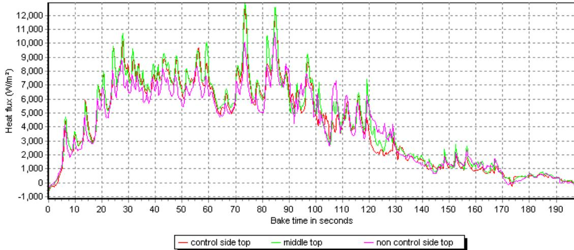
As the above graph shows there was a quite marked cross-band variation in top heat with more heat available on the centre of the band leading to paler, high-moisture product on each side of the band. This is a common problem on many multi-burner ovens even when fitted with tri-zone ribbon burners.
