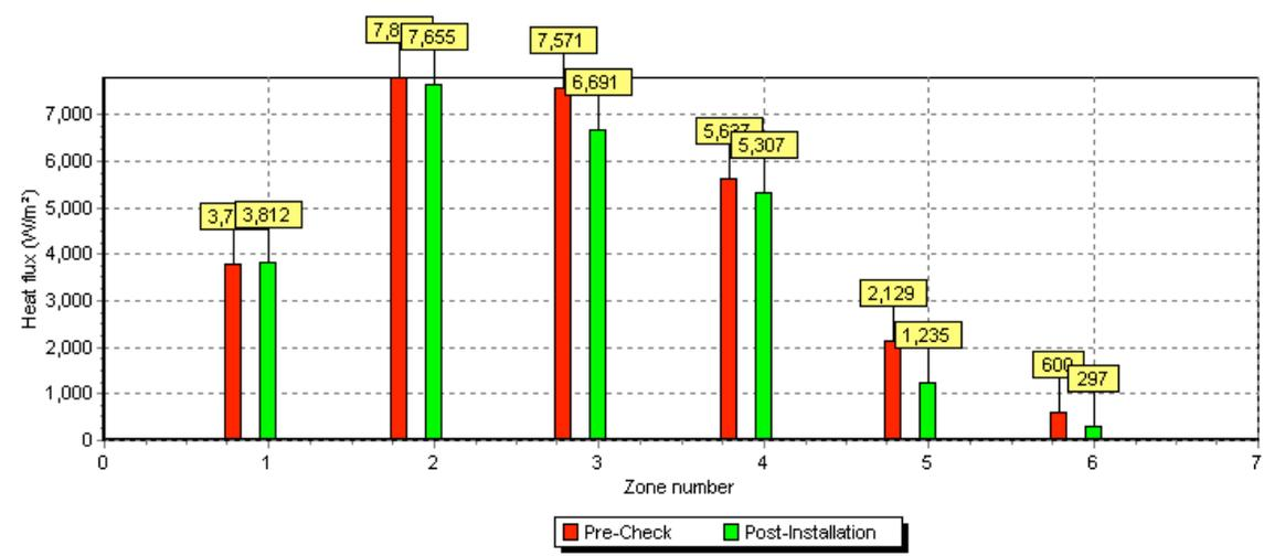
The heat profiles with the EnviroMont burner are noticeably different to the standard ribbon burners with a much “peakier” profile. These higher peaks are due to the extra radiant heat delivered by the incandescent Nitmesh behind the burner flame which also provides the efficiency improvement of the EnviroMont burner. However the potential negative impact of the higher peak is countered by the more significant dip in heat flux between the burners.
