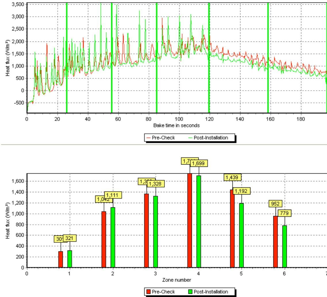
Overall both top and bottom heat profiles were reasonably well matched. Product quality parameters such as moisture and colour were also replicated. It should be noted that all the bottom burners in Zones 5 and 6 were off for both these audits and hence it was not possible to control and replicate the heat levels in these zones.
